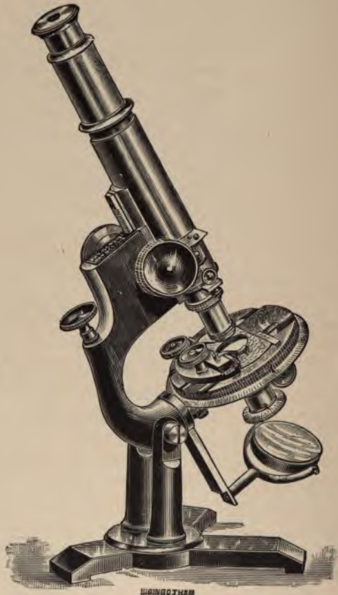
PETROGRAPHICAL MICROSCOPE. Made by Bausch and Lomb Optical Co., Rochester, N.Y. FIG. 47.
